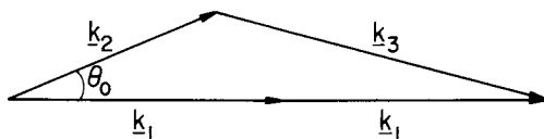
Figure 1. The phase-matching vector diagram for a CARS experiment. The length of each \kappa vector is n\omega/c where the refractive index is measured at frequency \omega at the subscripts on \kappa correspond to \omega_1, \omega_2 , or \omega_3 .
